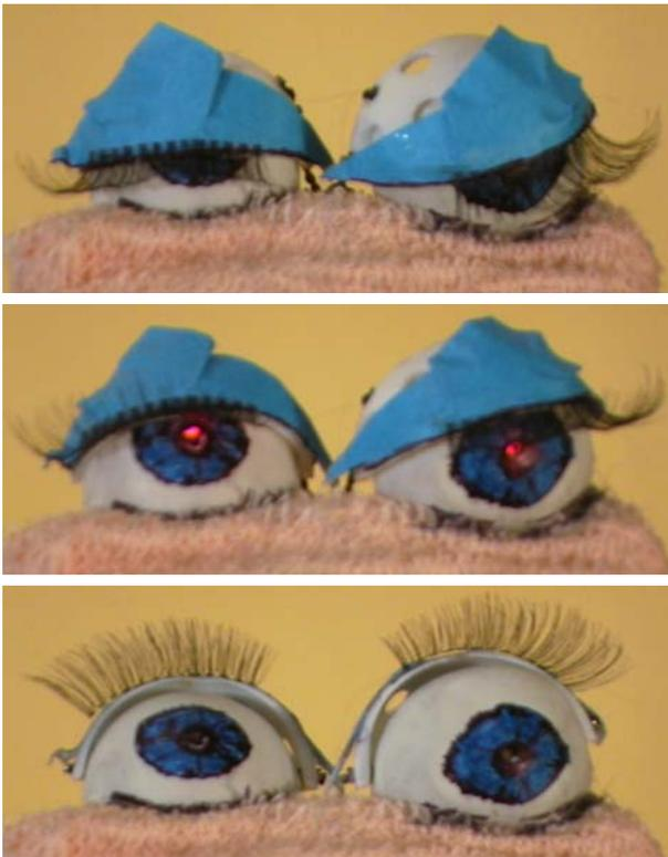
Figure 11: Phidget Eyes: closed, open & lit, fully open
