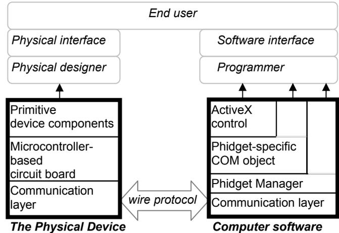
Figure 5. Phidget Architecture
