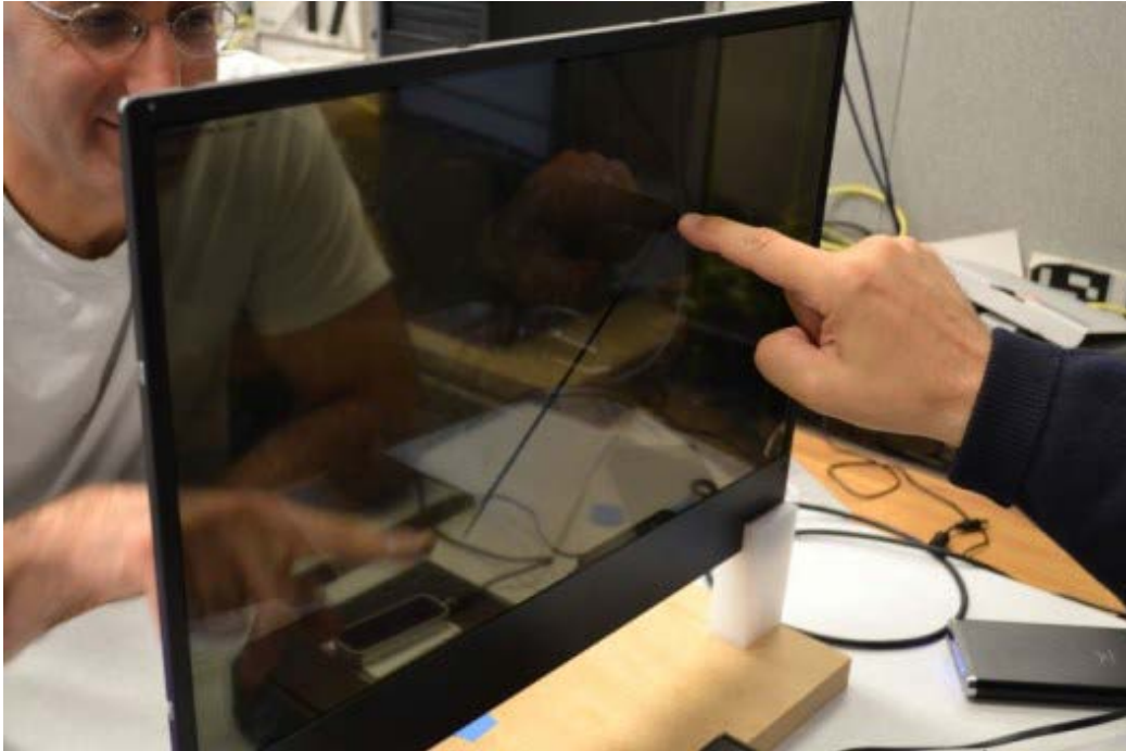
Figure 5. FacingBoard-1, our earlier transparent display allowing for two-sided input (here, simultaneous collaborative drawing) (Li, 2015).
