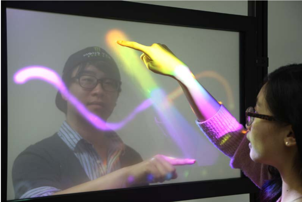
Figure 7. TransWall, a projection-based transparent display. The content on both sides was the same. (Heo et al. 2013). With permission from Woohun Lee.
