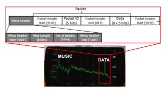
Figure 2: PhoneEar message template (the Hamming code is not shown in the diagram).
