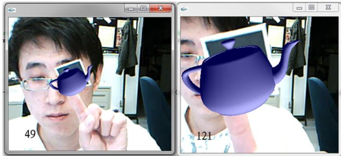
Figure 3-3: The software uses the tag width to estimate the distance between the tag and the camera.
