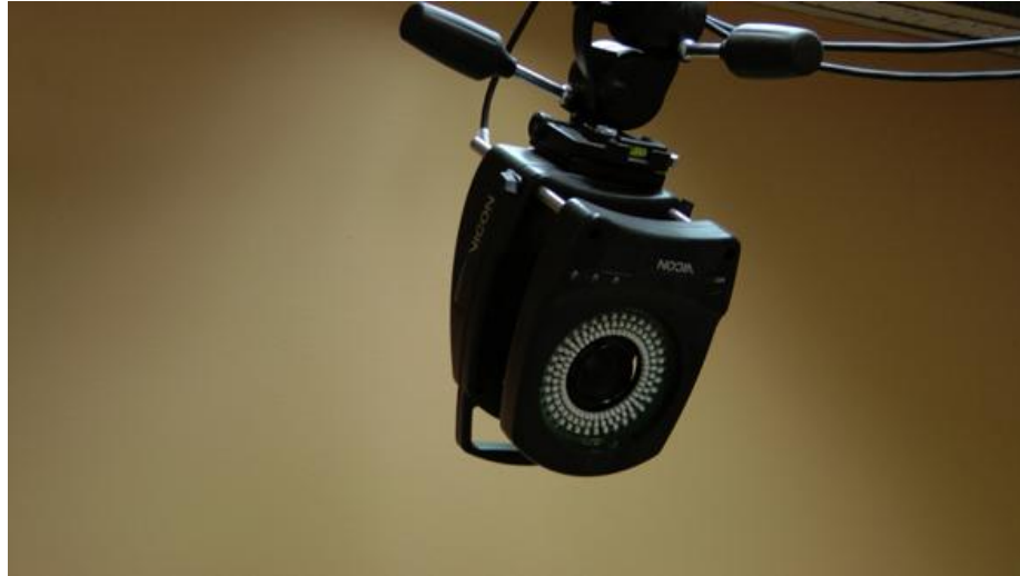
Figure 3-8: Vicon camera consists of an infrared camera in the middle and infrared lights around it.
