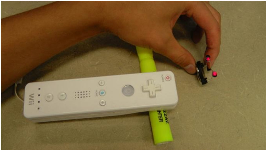
Figure 3-5: Wiimote and the infrared active marker.
