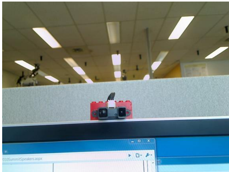
Figure 4-2: The infrared distance sensor sits on top of a computer monitor.
