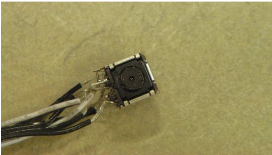
Figure 3-7: Wiimote's infrared camera.
