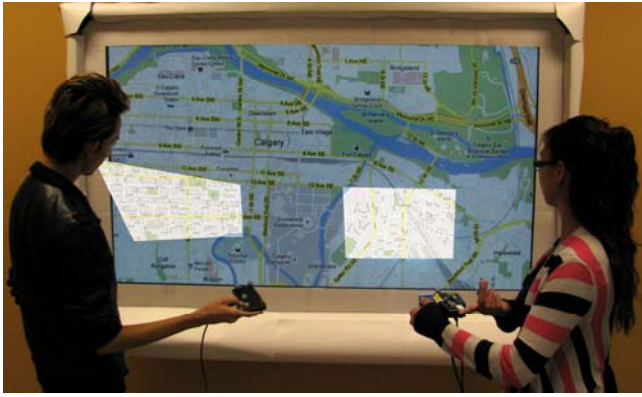
Figure 2: The map application. Two more detailed focus areas (one per user) are projected onto the stationary display. Projections are enhanced due to lighting issues.
