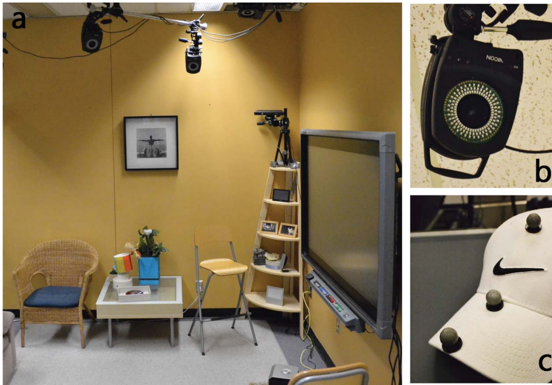
Figure 4-3. The Vicon Motion Capture System setup: a) the system tracks objects within a room-sized space; b) the infrared cameras targets at that space from different angles; c) reflexive markers are illuminated by the cameras, thus added to objects to represent their geometric structure and track their spatial presence..
