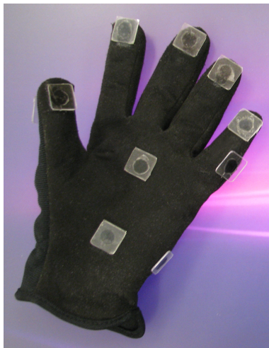
Figure 4.6: Fiduciary Glove with transparent tags.
