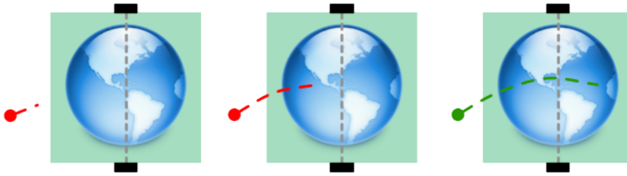
Figure 4.9: Example of gate activation: The gate is only activated in when the stroke (color dashed line) crosses the gate threshold (gray dashed line).
