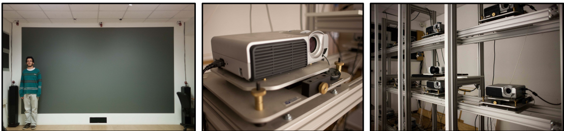
Figure 2.6: Left: Display size compared to average human height. Center: projector and calibration mechanism. Right: Support structure used to hold the 12 projectors.
