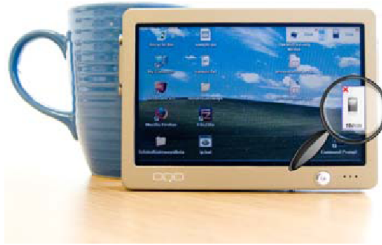
Figure 2.13: Hans Gellersen's Relate Gateways [18]: an icon on the screen spatially relates to a physical device
