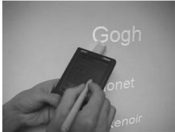
Figure 2.4: Text can be modified with the M-Pad device while holding it in close proximity [45].
