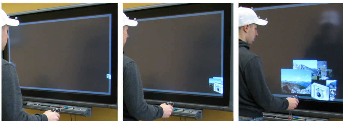
Figure 5.1: The camera symbol on the screen spatially relates to the physical device, gradually revealing photos and arranging them as a stack and then in a spiral, while coming closer.
