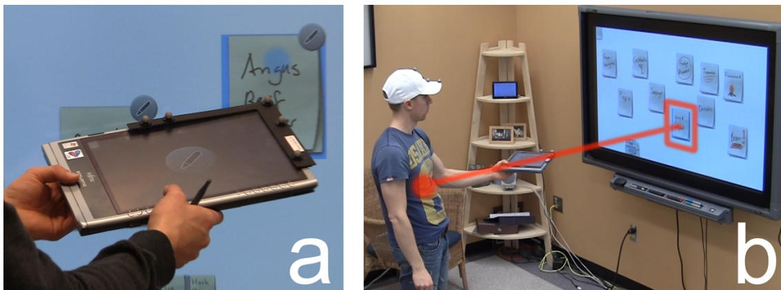
Figure 4.21: a) Holding the tablet in front of the large display shows a pointer and highlights the selected note before touching it for selection. b) Pointing from a distance to select a note. The red annotated line emphasizes the pointing direction and the highlighted sticky note.
