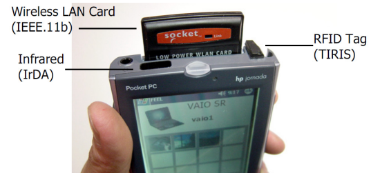
Figure 2.11: Rekimoto's M-pad is equipped with a RFID sensor for close interaction and an infrared sensor for distant pointing [47].
