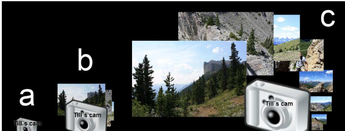
Figure 4.4: These three screenshots show how the camera gradually reveals its content while approaching the display from afar (a) to close (c).
