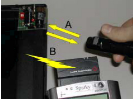
Figure 2.10: The GesturePen [59]: a pointing device with an infrared transceiver which can be used to select other devices.
