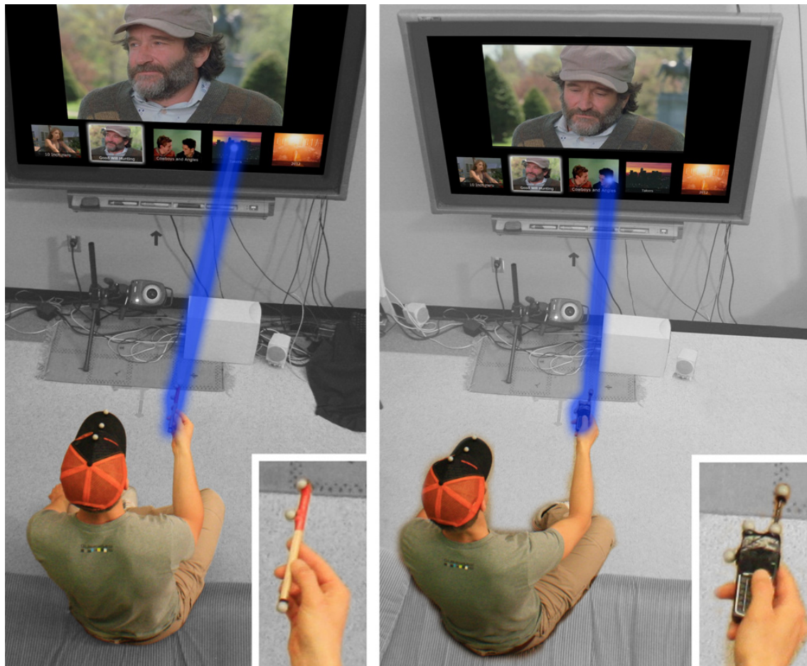
Figure 3.6: Explicit interaction triggered through distance and orientation between a person and a digital or non-digital physical artefact - left) a pen, right) a cell phone
