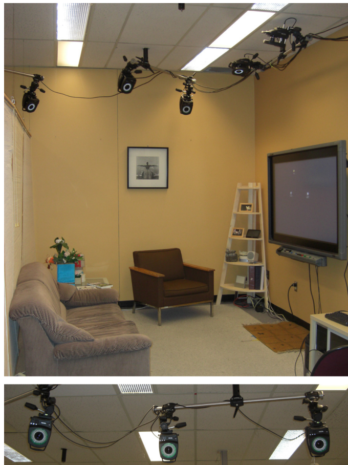
Figure 6.2: top) The prototyping environment as a living room setup with eight Vicon cameras mounted to the ceiling, bottom) three additional cameras are placed on the other side of the room.
