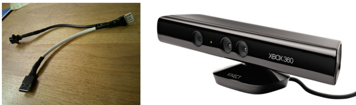
Figure 6.6: left) Custom USB-adaptor to connect a Kinect sensor with a computer, right) Microsoft's Kinect sensor [36]. Copyright 2010 Microsoft
