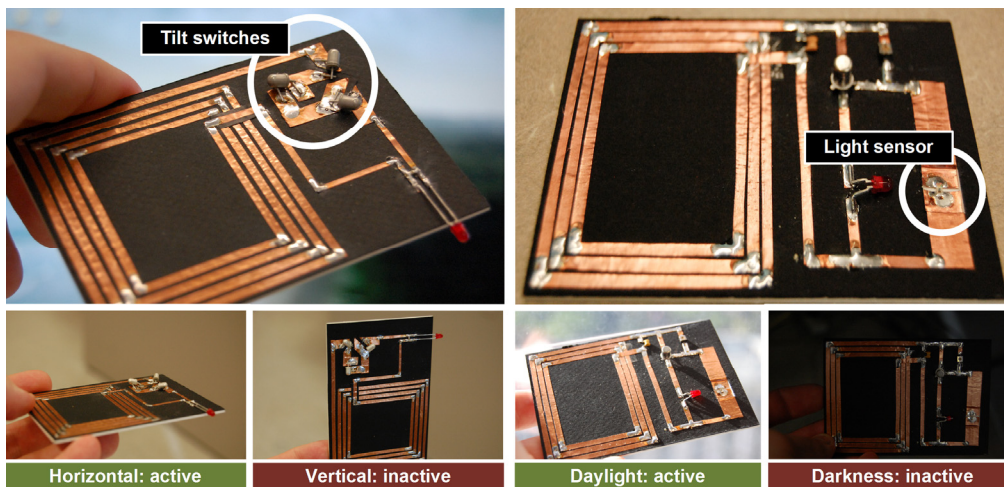
Figure 6. Tilt-sensitive (left) and light-sensitive (right) RFID tags.
