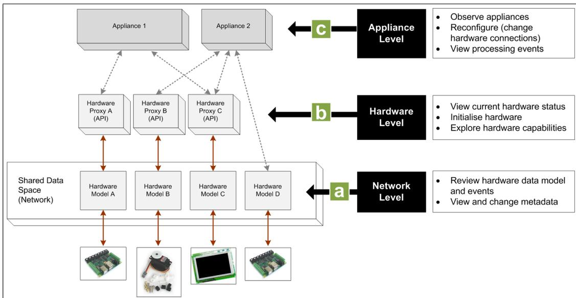
Figure 6.1: Three access levels to the shared infrastructure.
