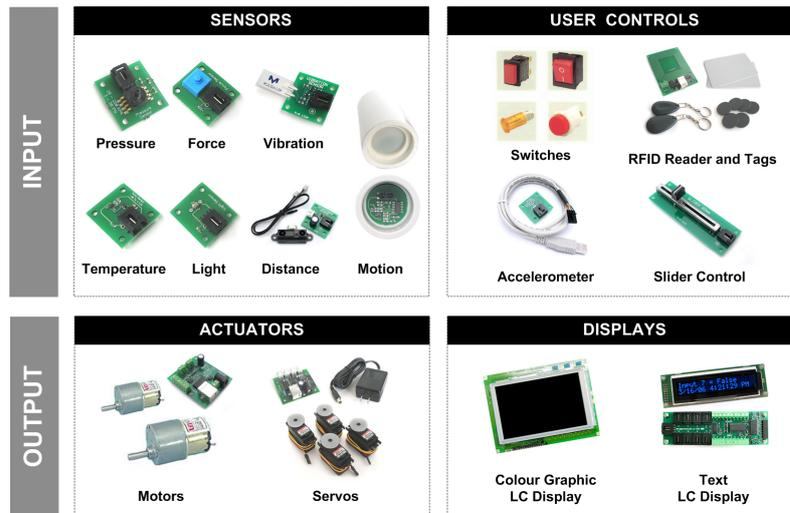
Figure 4.2: Overview of the physical user interface input and output components.
