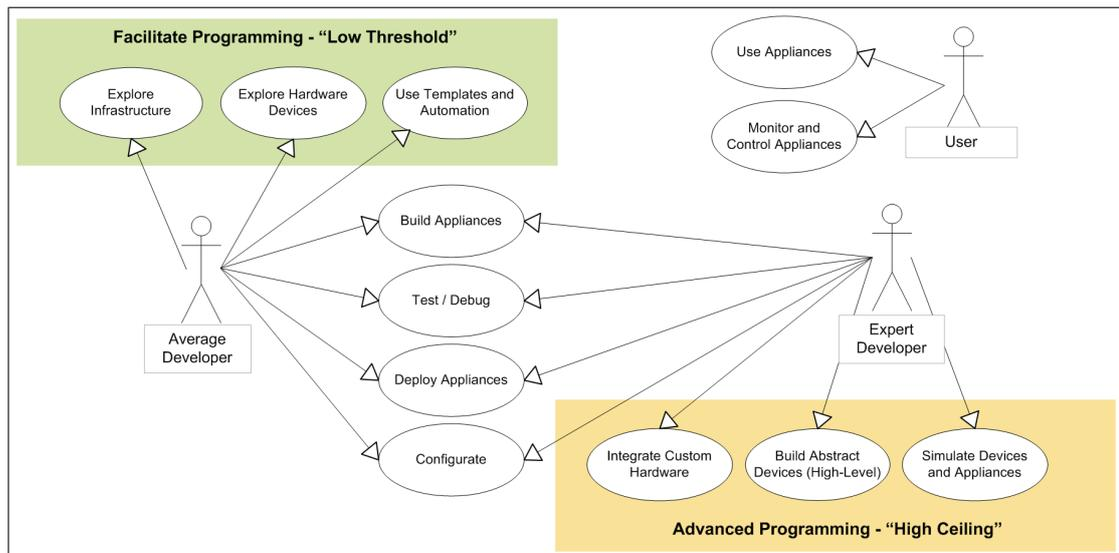
Figure 3.1: UML use case diagram.
