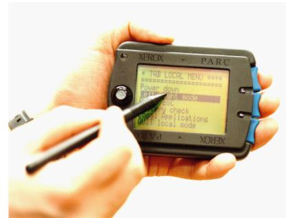
Figure 2.1: The tab prototype [Weiser, 1996].
