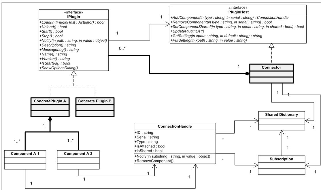
Figure 4.7: UML class diagram of the plug-in architecture.
