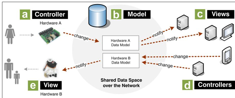
Figure 4.3: Distributed Model-View-Controller pattern.
