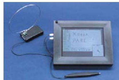
Figure 2.2: The paper sized pad prototype [Weiser, 1996].
