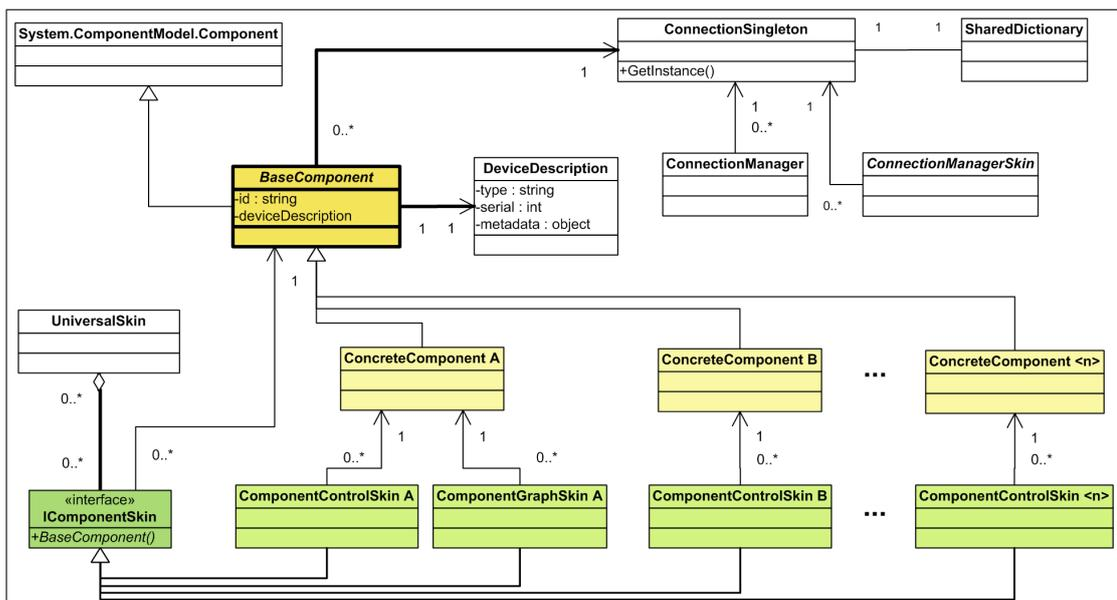
Figure 5.8: UML class diagram of the main components of the developer library.
