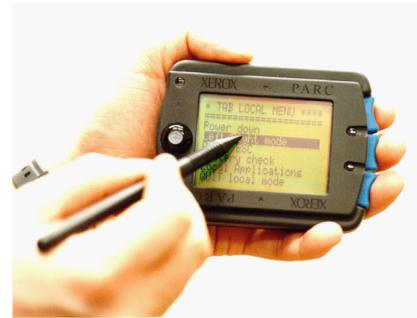
Figure 2.1: The tab prototype [Weiser, 1996].
