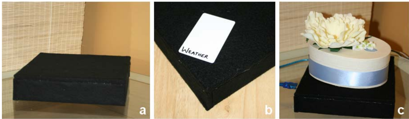
Figure 1. A smart location base, using an information card to assign a data stream to a location, and an appliance placed on a base.
