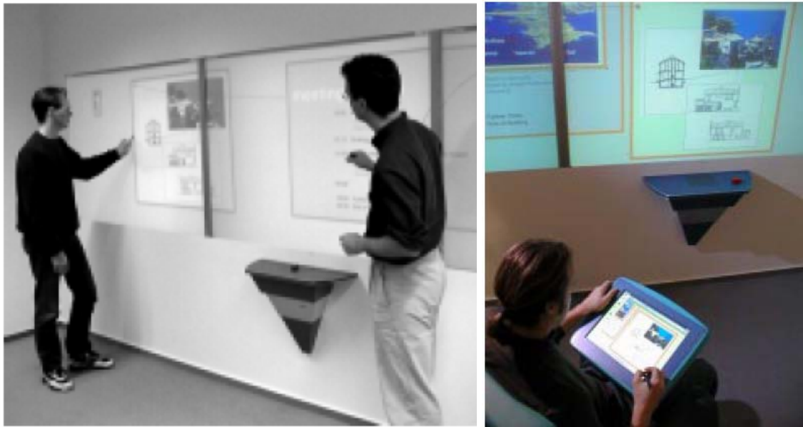
Figure 2.1 The i-LAND room: Collaboration on a wall display, and remote annotation from a CommChair to the wall [Reproduced from Figures 2 and 5, in Streitz, 1999, page 124].
