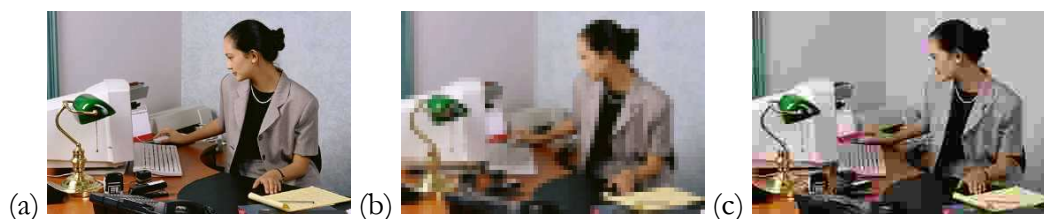
Figure 2.4 Bandwidth requirements of high-quality video (a) can be reduced by decreasing the number of pixels in an image (b) or by using compression (c), but these methods affect social transparency.
