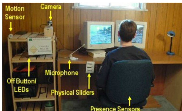
Figure 10.1—The Home Media Space prototype included environmental sensors that were used to autonomously enable/disable capture. The camera was mounted on a servo motor so that it could be rotated to face the room or face the wall. (Figure reproduced from Neustaedter & Greenberg, 2003.)
