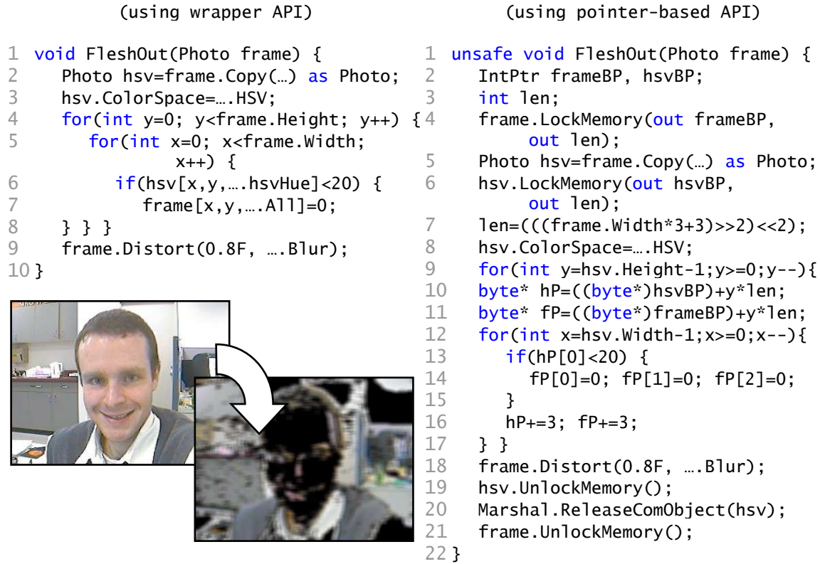
Figure 3.8—Custom video analysis/manipulation technique to remove flesh-coloured pixels.
