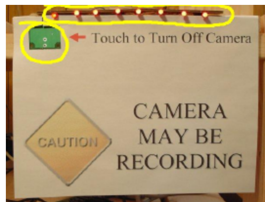
Figure 6.11: A sign containing LEDs (circled at the top) and an off button (circled below the LEDs).
