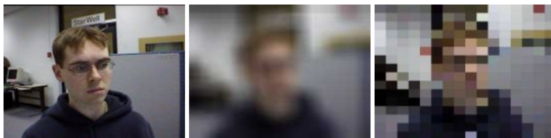
Figure 1.3: An unfiltered media space view, the view with a blur filter, and the view with a pixelized filter.
