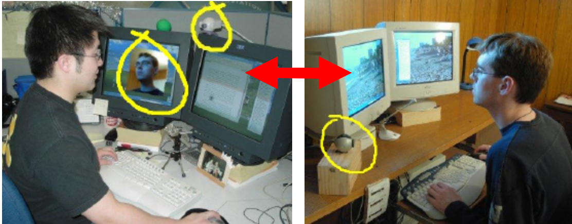
Figure 1.2: A typical video media space where video is used to provide informal awareness between distance-separated colleagues. PC cameras (circled) capture each collaborator and this information is broadcast to the other colleague (circled on the display of the person on the left).
