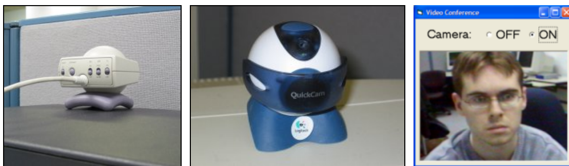
Figure 2.3: Three example “pull the plug” mechanisms for controlling privacy: turning the camera to face a wall (left), flipping down a plastic visor (middle), and toggling a software control (right).
