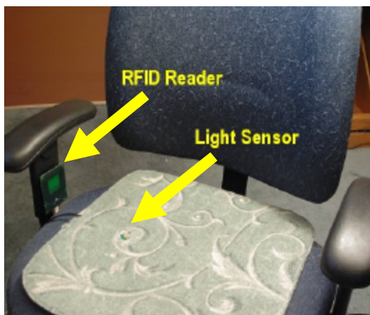
Figure 6.12: The RFID reader and light sensor to detect the telecommuter's presence.
