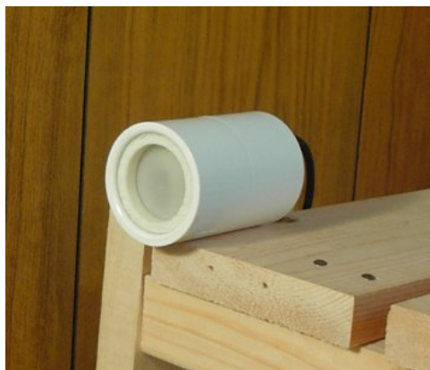
Figure 6.14: The infrared motion sensor used to detect the presence of people in the home office/spare bedroom.
