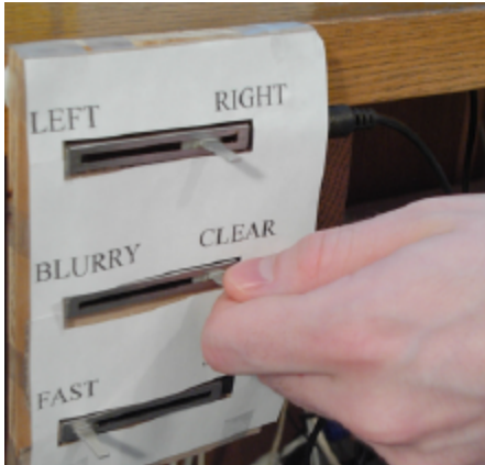
Figure 6.8: A user adjusts the blur level with a dedicated physical slider.
