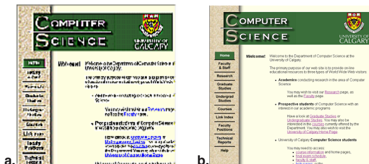
Figure 5-9. Comparing (a) row and column deleting algorithm with (b) box filter.
