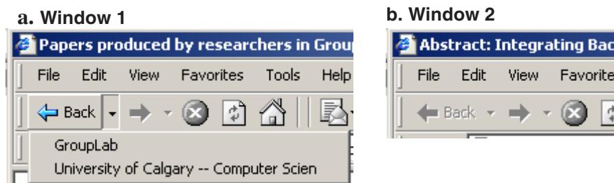
Figure 5-1. Pages visited in Window 2 are not accessible from Window 2 via back/forward. Also, the page in Window 2 is not accessible in Window 1 via forward.
