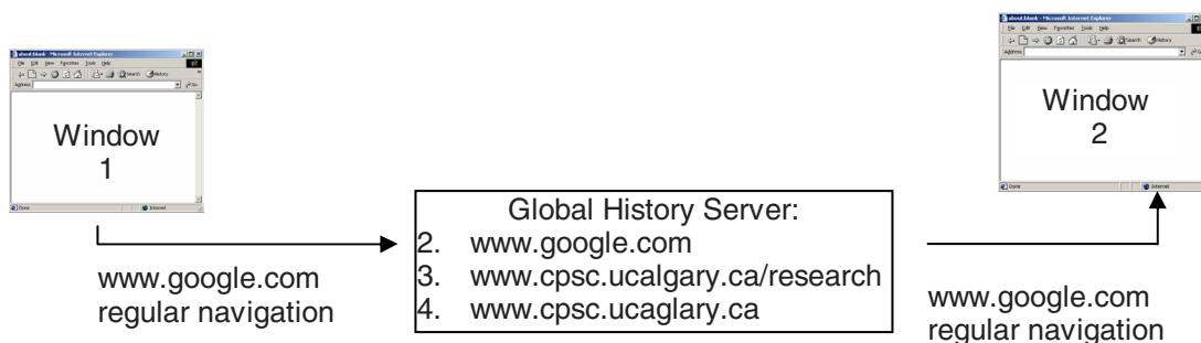
Figure 5-3. When the user navigates in Window 1, the window communicates the event to a server process that passes it on to the other windows.
