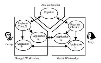
Figure 3. Basic run-time architecture of GroupKit.
