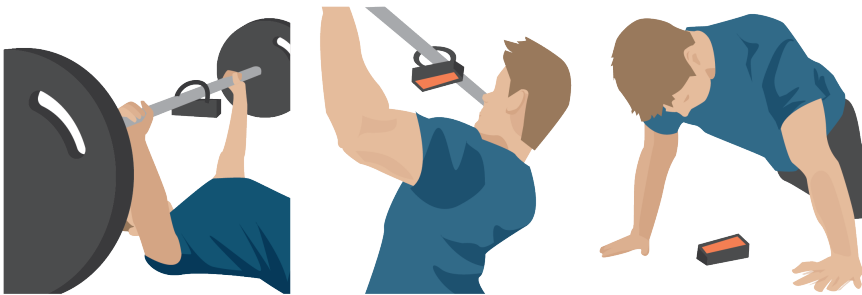
Figure 7.1. Gymbuddy (by Mike Chubey) is a mobile device which can be attached to gym equipment (e.g., bench press) and provides training and assistance through the display. The system keeps track of repetitions via a distance sensor.
