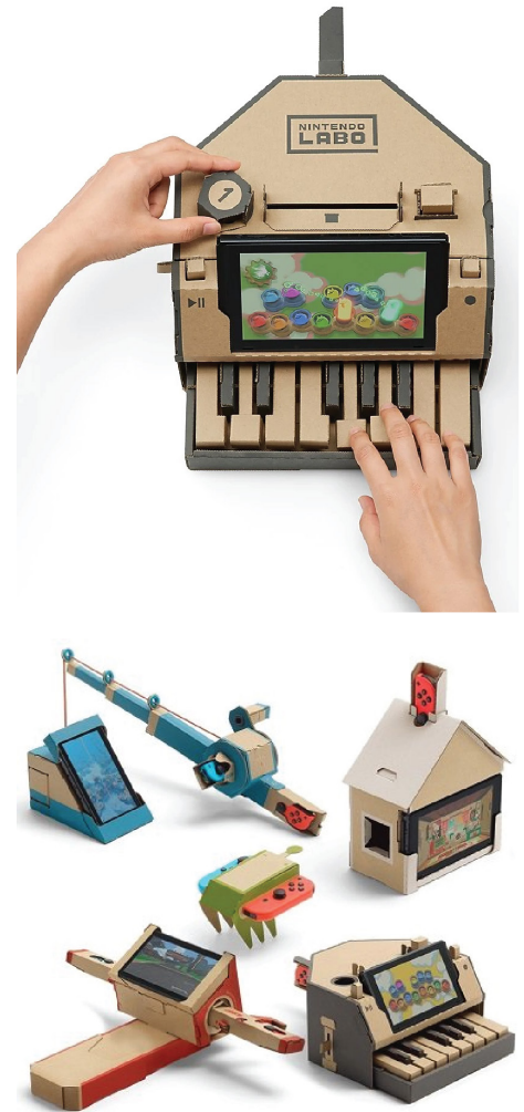
Figure 6.1. Nintendo Labo from 2018 enables players to insert the Nintendo Switch tablet and controllers into cardboard enclosures. Different controller sensors (e.g., the IR camera) are used to sense user input as defined by the enclosure.
