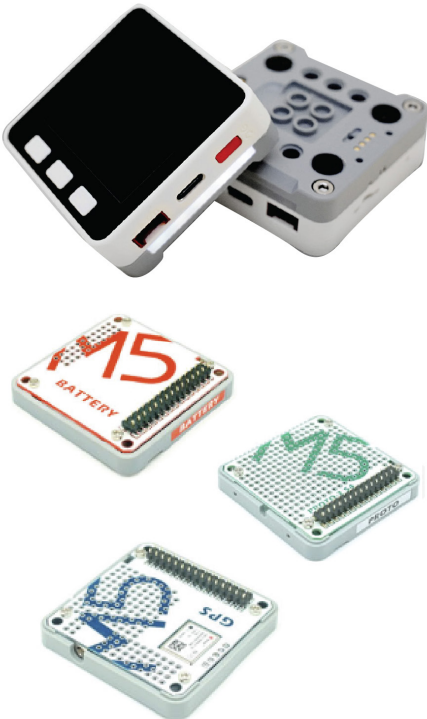
Figure 6.2. M5Stack device. The image shows the M5Stack base module featuring a 2 inch x 2 inch touchscreen, 3 buttons, USB port, and a Lego-compatible peg at the bottom to attach other modules. The bottom three images show the modules for battery, prototyping and GPS. Image adapted from http://www.m5stack.com/
