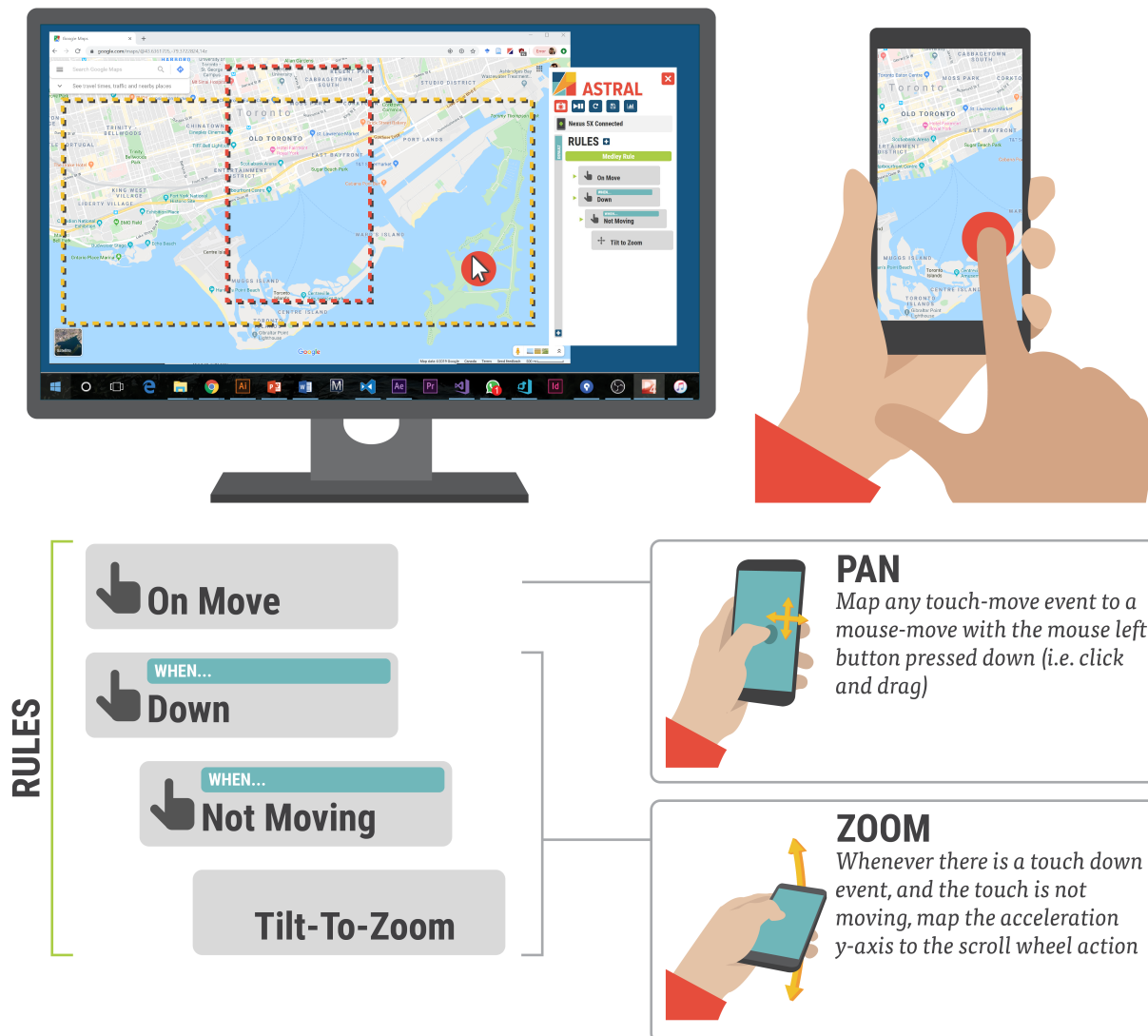
Figure 9.12. Tilt-to-Zoom Prototype. This figure shows how Astral leverages conditionals to create an interaction that requires considerable coding only repurposing a web browser on the desktop.
