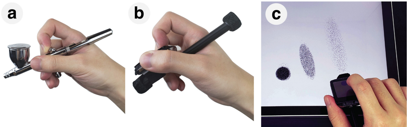
Figure 7.8 Physical airbrush (a), and its replication in WatchPen (b) which can control the ink flow with the watch's touchpad. The orientation of the pen (c) changes how the paint is spread on the canvas.
