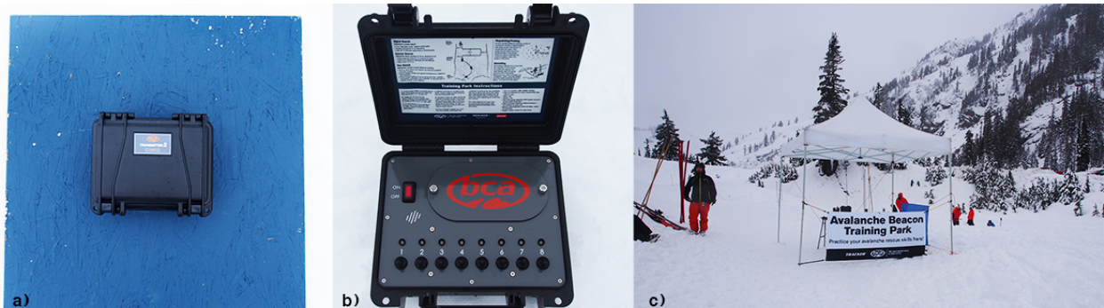
Figure 1. a) Practice beacon in waterproof case on plywood. b) Beacon park control box. c) Beacon park area.
