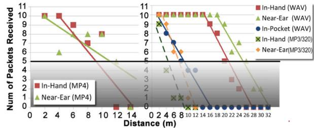
**Figure 4: Number of received packets using MP4 video (left), and WAV and MP3 (320kbps) audio formats (right). The black line represents half of the sent packets.**
