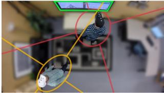
Figure 2. The Proximity Toolkit gives precise information about each person's position and orientation relative to each other and the display.
