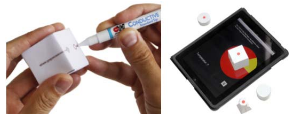
Fig. 4 Sketching conductive ink on a Paperbox object (left), and then using it to interact with a tablet (right).
