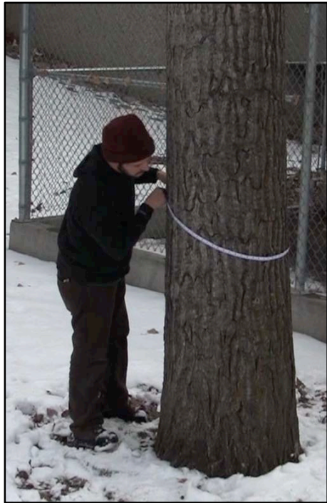
Figure 4. Steve lets his tape sag, which produces erroneous readings.
