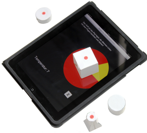
Figure 4. A working Sketch-A-TUI prototype showing the graphics it is controlling on an iPad.
