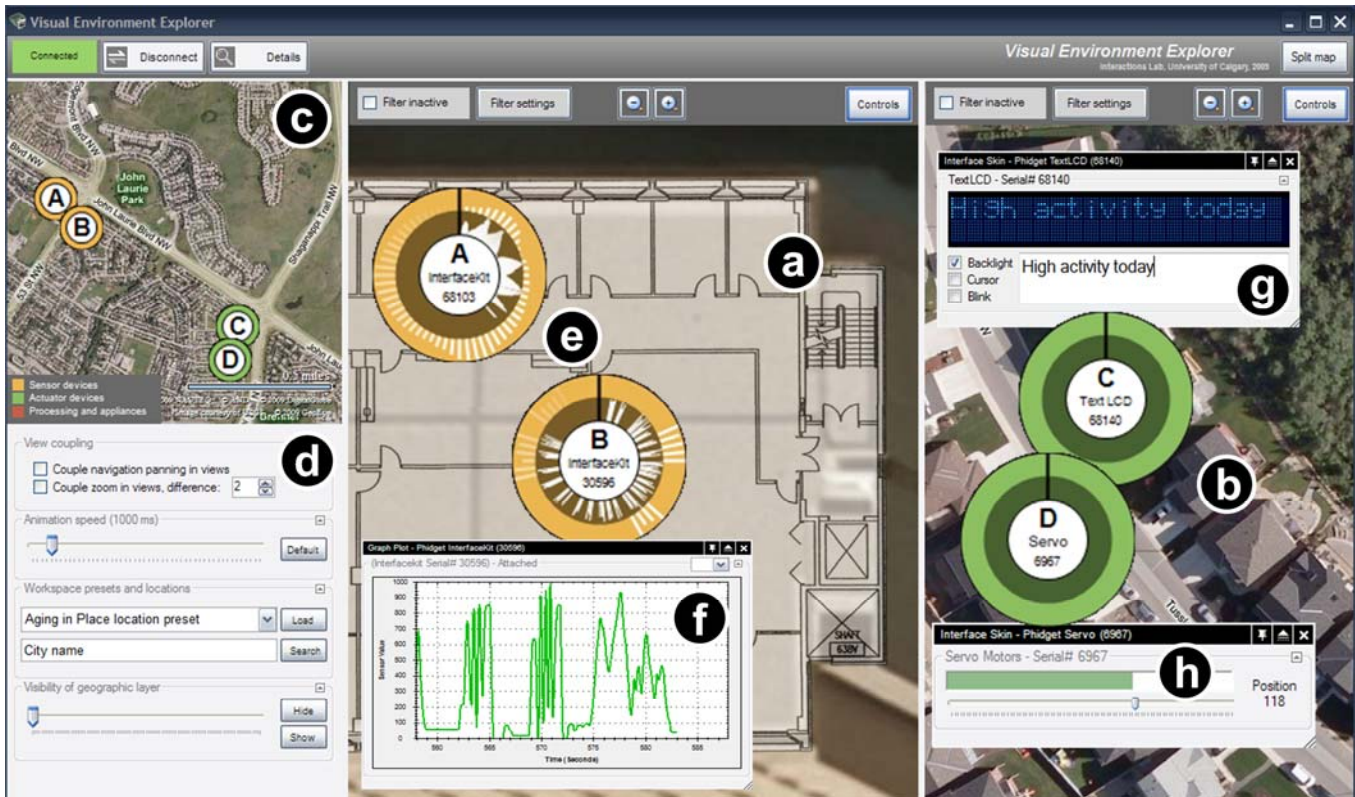
Figure 2. The VEE user interface: visual exploration of distributed sensors and actuators.
