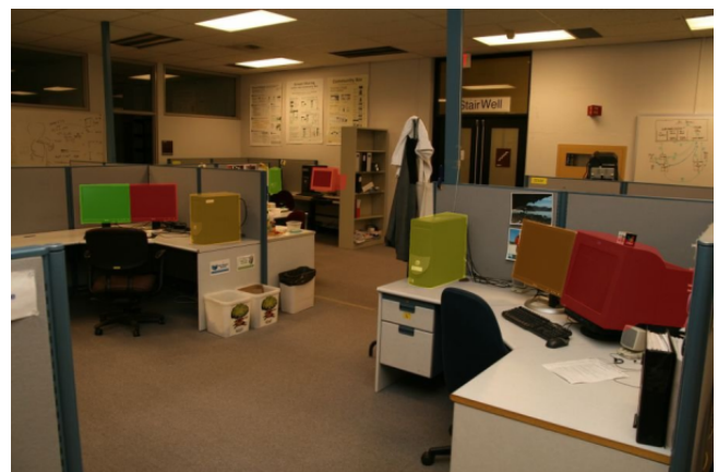
Figure 1. HomeWindow showing the energy usage of several monitors, displays, and computers with colored auras. Red is high usage while green is low usage.
