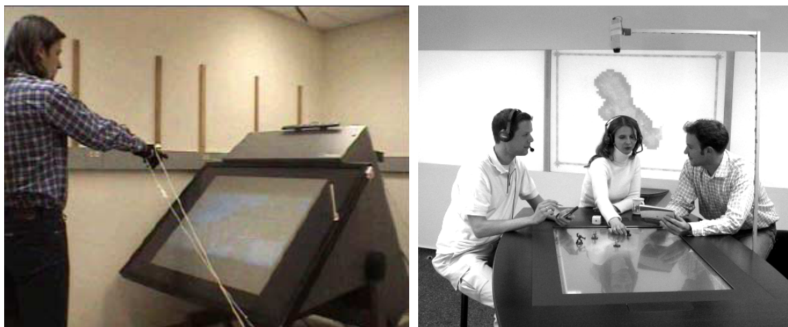
Figure 2.24. Alternative display form factors for multimodal interaction: a drafting board orientation from Corradini et al. , 2002, a tabletop surface from Magerkurth et al. , 2004.
