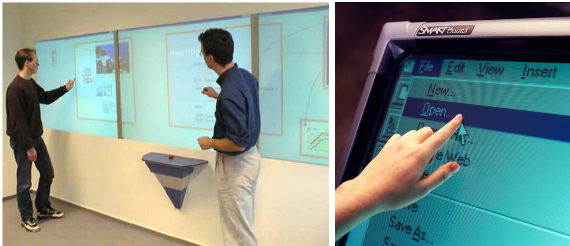
Figure 2.5. Multi-touch wall displays: Multiple tiled Smart Boards in the Dynawall from Streitz et al. , 1999 (left) dual touch DViT (right), from www.smarttech.com
