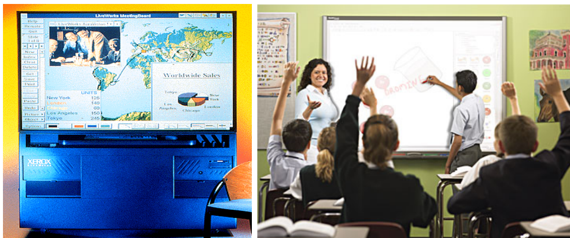
Figure 2.4 Single point interactive wall displays: Xerox Liveboard, Image courtesy of Palo Alto Research Center, photographed by Brian Tramontana (left), single touch analog resistive Smart Boards from www.smarttech.com (right)
