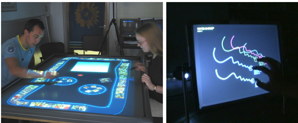
Figure 2.12. Infrared touch sensing technologies: DVIT Smart Board, from Hinrichs et al. , 2005 (left) FTIR sensing, from Han, 2005 (right)
