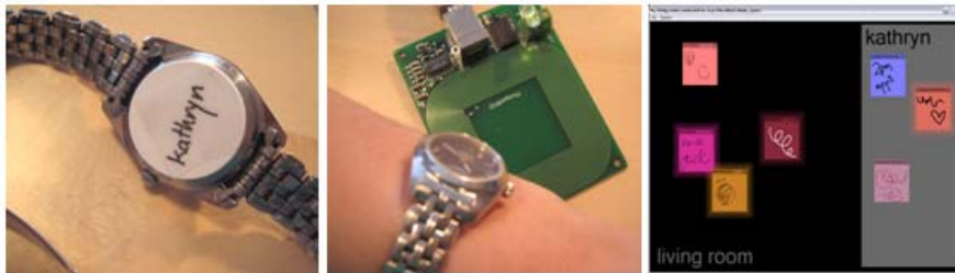
Fig.6: RFID tags, small enough to be worn, identify people, and show them personal messages.
