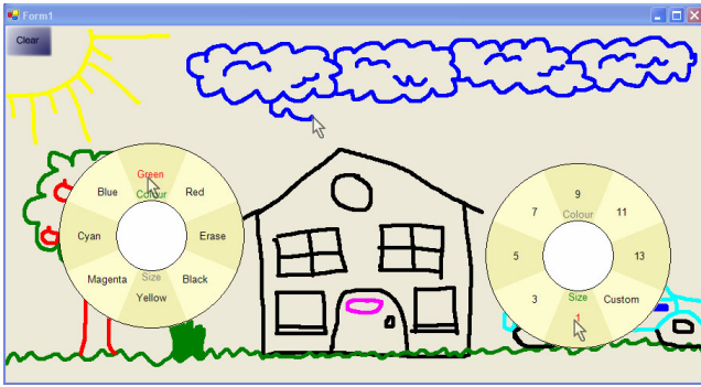
Figure 7. An SDG drawing application. Two users are select a drawing color and size from their individual flow menu, as the third is drawing.
