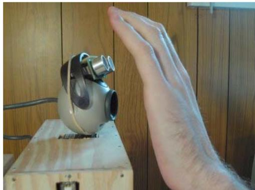
**Fig. 9.** A user blocks the camera with his hand to turn it off.
