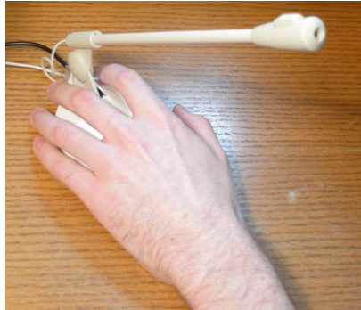
Fig. 10. A user moves his hand over the microphone to open an audio link.
