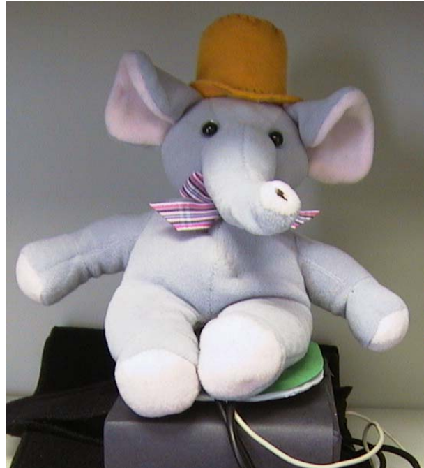
Ele-Phidget by Shivaughan Warwaruk is an ambient notification for an audio chat program. When you receive a message, the elephant turns around and faces you. You push the elephant's stomach to listen to the message. When no messages are left, the elephant turns away. To record a message, you squeeze the elephant's head and speak into the elephant's trunk. A second squeeze sends the message.
