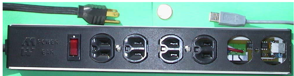
Figure 3: GlabPowerBar. Note the USB connection and the circuit board just visible inside
