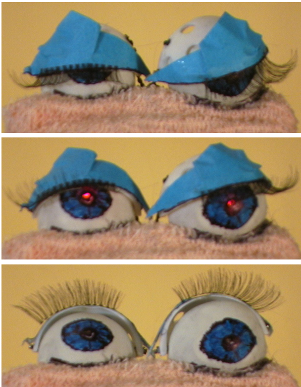
Figure 11: Phidget Eyes: closed, open & lit, fully open
