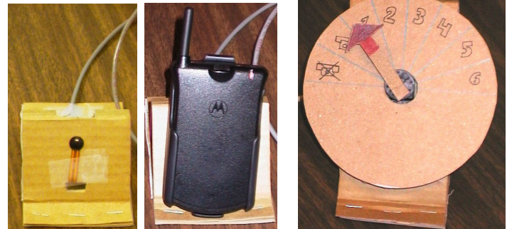
a) cradle b) cradle & phone c) missed calls dial Figure 12. Missed Calls
