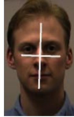
Figure 5. Visualization of the face position, dimensions, and orientation information output by the CAMSHIFT algorithm.
