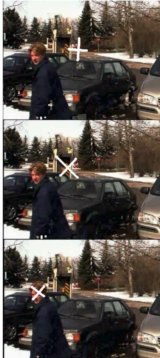
Figure 14. Frame at which track was lost under (from top to bottom) the 1 fps, 5 fps, and 10 fps frame rate conditions.
