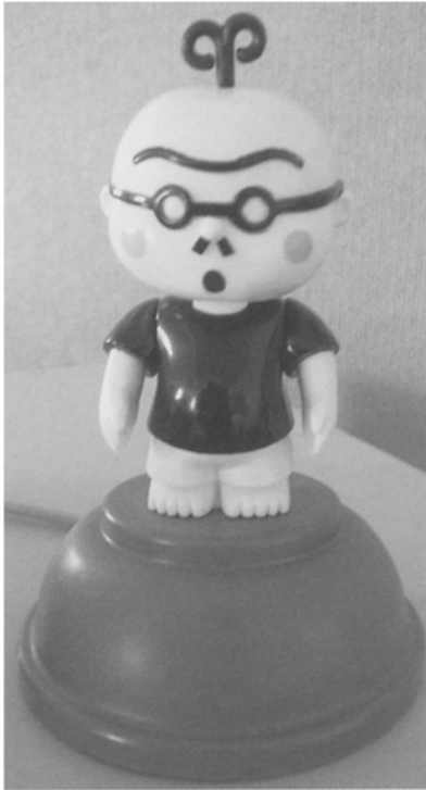
Fig. 6. The Fujitsu device. Through programming, a red and green light in its head can be turned on and off; its hand and head can be raised or lowered; and we can detect when its head is pressed.
