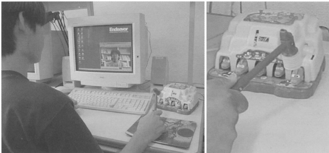
Fig. 8. A multi-user awareness surrogate, where each alligator represents a different person, and their movement in and out of the cave indicates that person’s availability. Hitting the alligator with a hammer establishes a video connection between the two.
