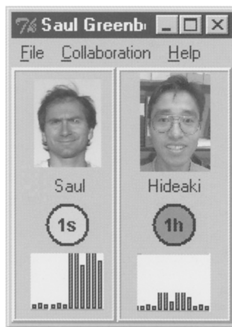
Fig. 1. Our iconic indicator. Images fade as the remote person's interest in the local person decreases [9]. Lights indicate by colour [10] and text how much time has passed since the person last touched their computer. Bar charts graph the degree of a person's motion over time e.g. Saul has recently entered his office, while little activity has been seen in Hideaki's office.
