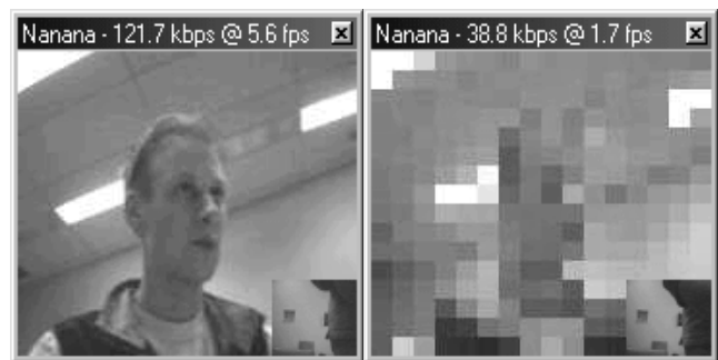
Figure 4. Highest and lowest qualities of service offered in our video media space app. Utilizes the pixelize filter.
