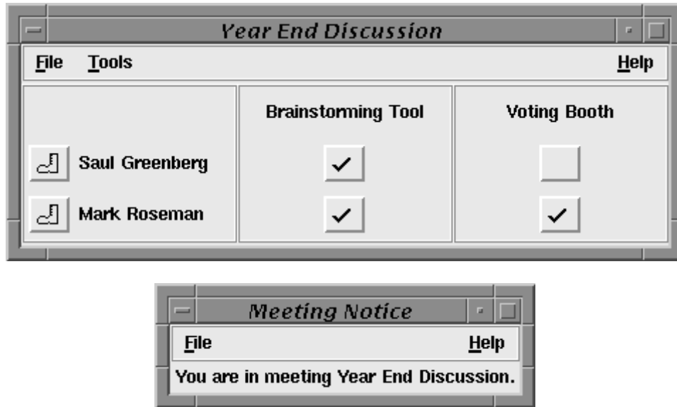
Figure 11. The Centrally Facilitated session manager. The Facilitator's control panel for managing sessions is shown on top. Participants just receive a notice that they are in the meeting.
