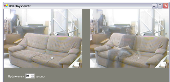
Figure 2: Motion blur visualization applied with an update rate of once every ten seconds. The visualization on the right shows ghost images of the subject in different areas of the space.
